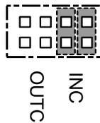
When using the INC jumpers, the digital inputs must have a reference. This reference comes from the RIO from pin34 (INC0B) for inputs 0-7 and from pin 16 (INC1B) for inputs 8-15.
