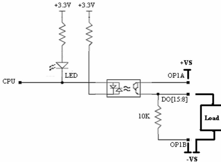
OP1A should be connected to the positive side of 5-24VDC external power supply.
