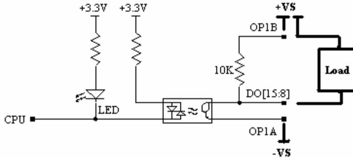
OP1B should be connected to the positive side of a 5-24VDC external power supply.
