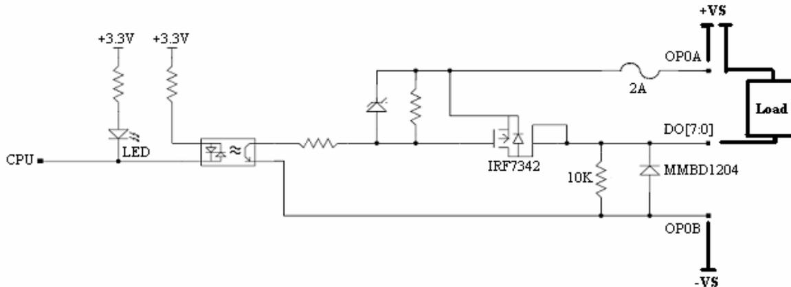
OP0A should be connected to the positive side of a 12-24VDC external power supply.
